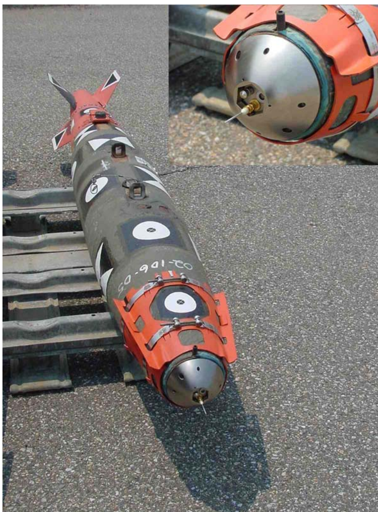
Figure 2: Weapon Separation 6 DoF Unit in 500 lb JDAM
