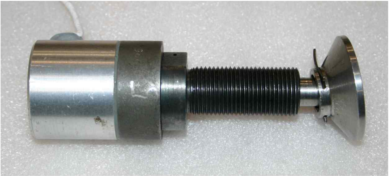
Figure 12: External Load Cell mounted on BRU-36 Sway Brace Pad
