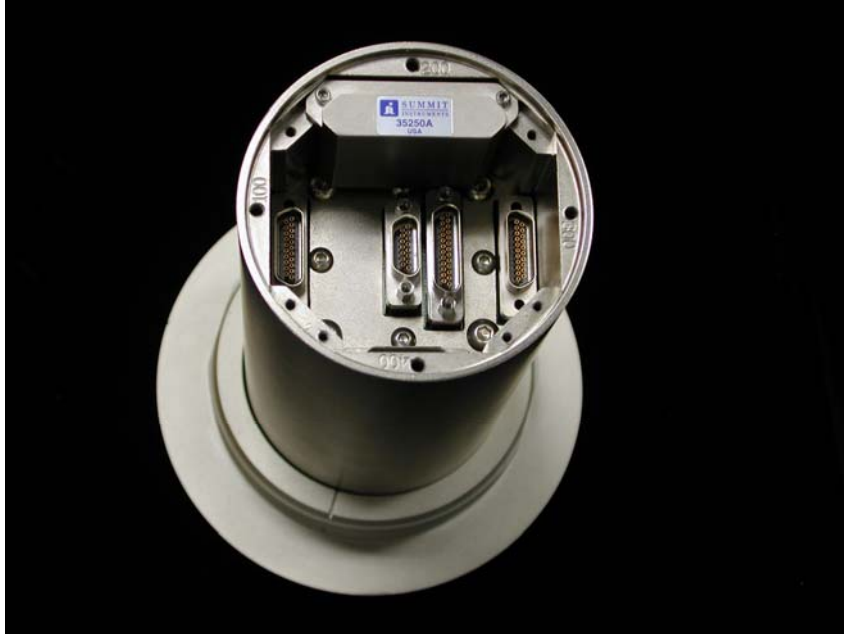
Figure 9: Interface for external instrumentation on Captive Carriage Miniature Telemetry Unit
