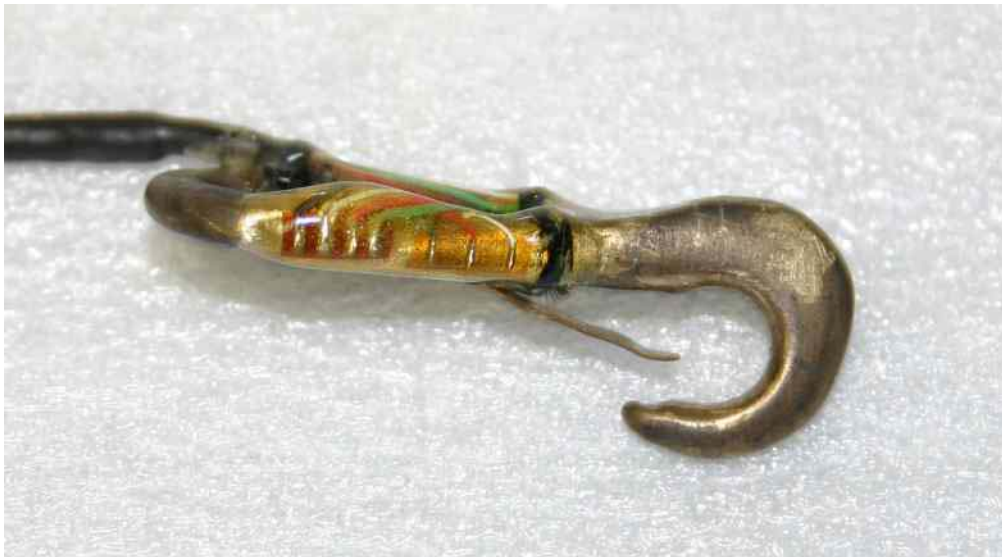
Figure 6: External Strain Gauges mounted on AV-8B Umbilical Lanyard release hook
