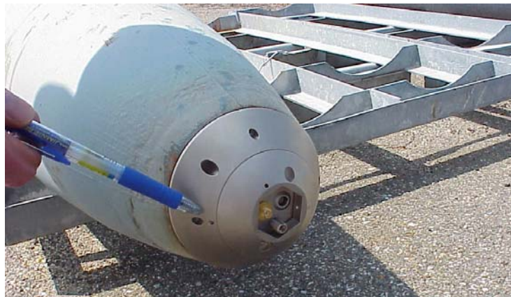
Figure 8: Captive Carriage Miniature Telemetry Unit installed in MK 80 Series Store
